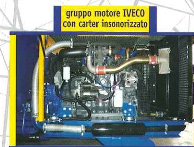
IVECO engine with sound-proof casing
