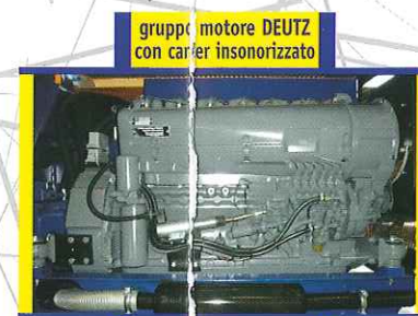
DEUTZ engine with sound-proof casing
